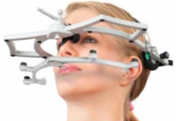
FIG. 2 — The Jaw Motion Tracker (JMT) by SICAT allows for a patient’s functional movement tracings to be recorded digitally and to be evaluated in 3-D with CBCT image.
