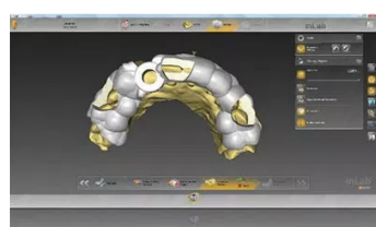
FIGURE 13. The software displays a proposal of the surgical guide, with the option of using various tools to modify the design (for example, by the integration or removal of viewing windows).
