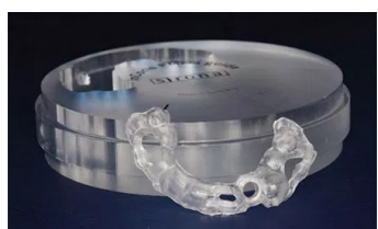
FIGURE 14. Removal of the surgical guide from the milled disk.
