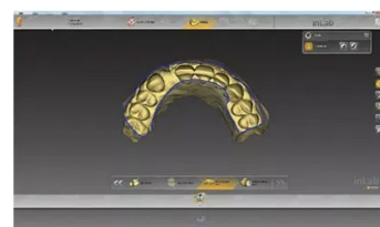
FIGURE 10. The laboratory trimmed the digital model of the implant surgical guide directly in the software.
