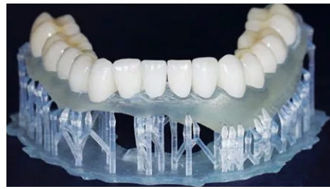
FIGURE 4. Prosthetics fitted on a stereolithography printed model; note the precision of the restorations produced using computer aided design/computer aided manufacturing technology.
