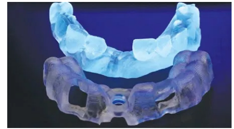
FIGURE 5. Printed model and a surgical guide milled using computer aided design/computer aided manufacturing equipment.
